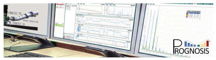
This platform is able to retrieve data from SCADA/PLC already available on the asset, via the most common industrial protocols (**ModBus**, **OPC UA/DA**, etc.). Moreover, it is possible to acquire signals from additional instrumentation installed for the task, such as vibration sensors.
