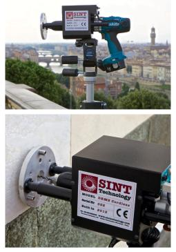
The Drilling Resistance Measurement System (DRMS Cordless) is a useful portable tool that continuously measures the force required to drill a hole in the investigated material during all the testing process. This parameter is called **Drilling Resistance** and it can be measured by drilling a hole with a suitable drill bit (usually with a diamond tip) on many different materials, mainly **natural stones**, **rocks**, **mortars and bricks**.
