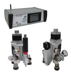
The MTS3000-Restan system is an **automatic measurement chain** for hole-drilling residual stress measurements: the full control of the device during the drilling and the acquisition process guarantees high accuracy of the results and reduction of the measurement uncertaity connected with the measurements.
