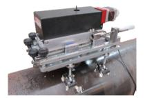
The software allows also the acquisition of the digital camera installed on the mechanical body of the device: this camera is used for the centering the strain gage with the drilling axis thanks to the presence of two laser beam that are able to project two perpendicular lines directly on the tested workpiece. These lines can be aligned with the strain gage reference positioning lines.
