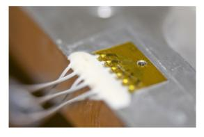
The hole-drilling method allows accurate experimental stress analyses at moderate costs. It consists in drilling a small hole (typically 1.8 – 2.0 mm) which changes the initial deformation allowing redistribution of residual stresses locked in a material.
