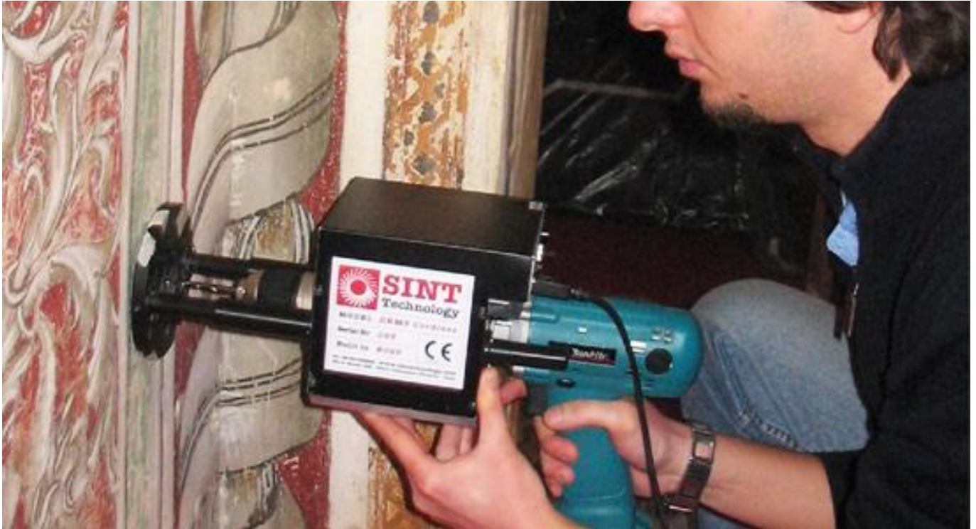
Drilling Resistance tests in the Santa Croce Basilica (Florence)
